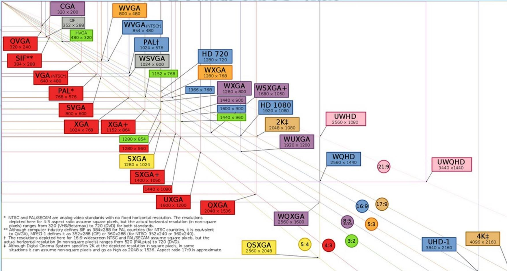
\* NTSC and PAL/SECAM are analog video standards with no fixed horizontal resolution. The resolutions depicted here for 4:3 aspect ratio assume square pixels, but the actual horizontal resolution (in non-square pixels) ranges from 320 (VHS/Betamax) to 720 (DVD) for both standards.
